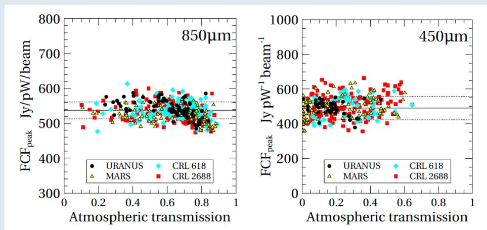
The error on the relative flux calibration is less than 5% at 850 $\mu$ m and  $\sim$  10% at 450 $\mu$ m. **A factor of 2 improvement over SCUBA.** Mostly due to the use of a line of sight water vapour meter.
