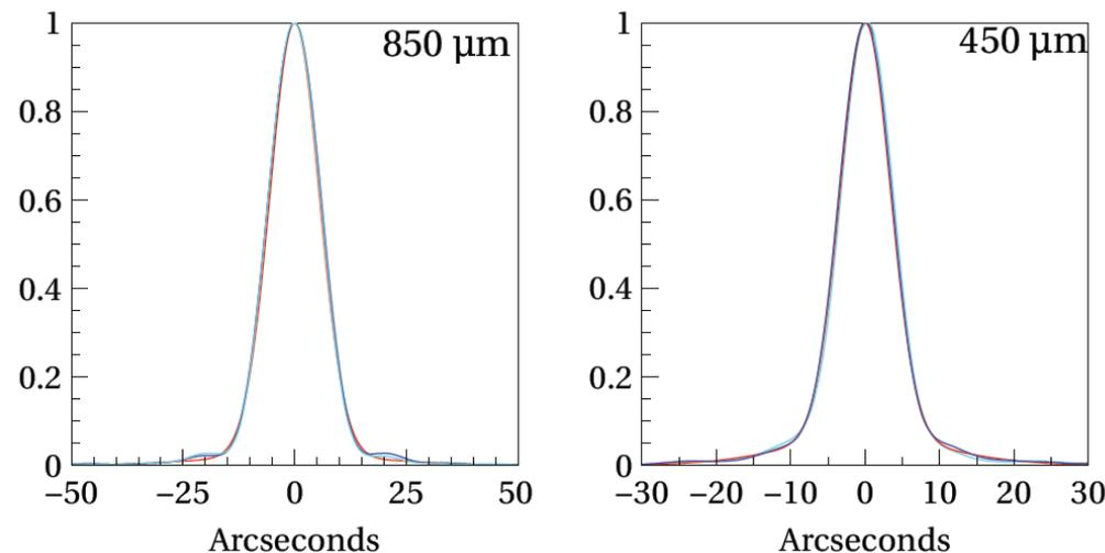
Measured the SCUBA-2 beam shape and focal plane distortion to enable accurate aperture photometry.
