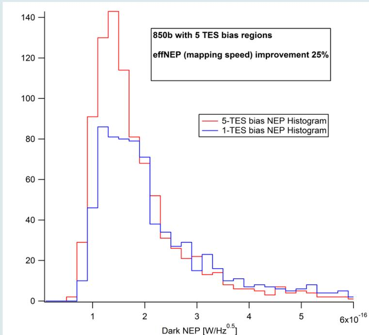
Multiple TES biased regions could improve the mapping speed of 850b and 850d significantly.
