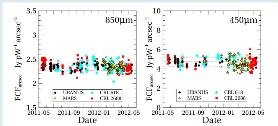
**Calculate a Flux Conversion Factor (FCF) from detector units (pW) to astronomical units (Jy).**
