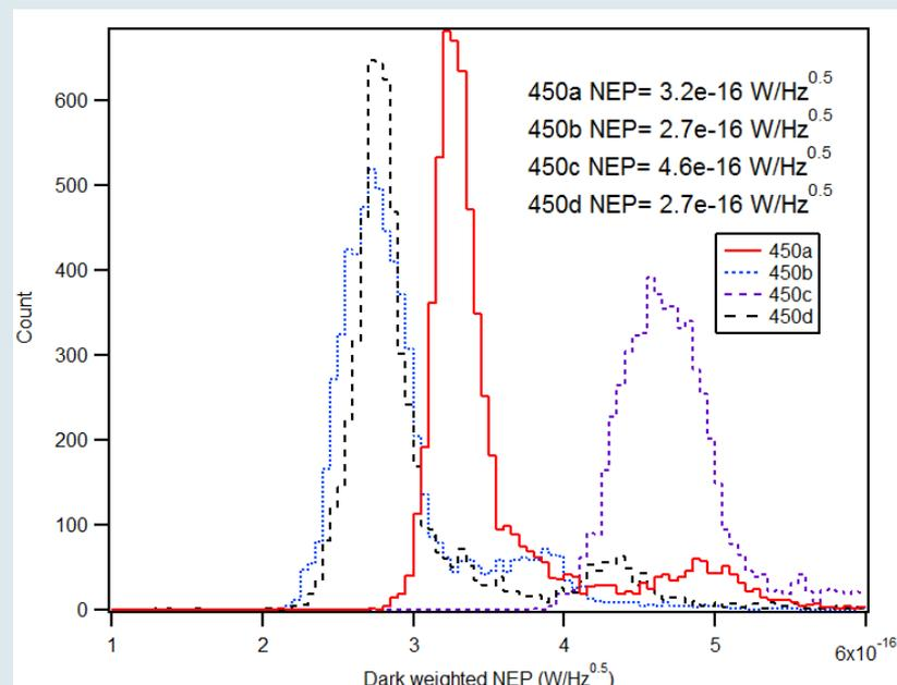
Dark NEP histograms for each sub-array; (right) 850 focal plane (left) 450 focal plane. These comprise all the dark noise observations from Feb 2012 to June 2012: 6,500 NEP measurements in total. **The measured dark NEP is higher than the expected phonon noise limited NEP.**
