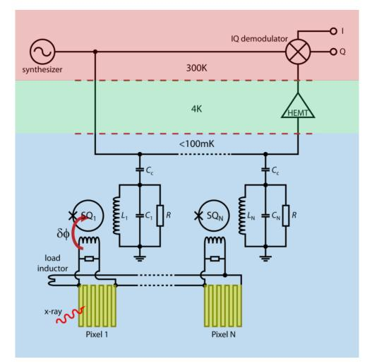
single HEMT and two coaxes for readout of ~1000 detectors
