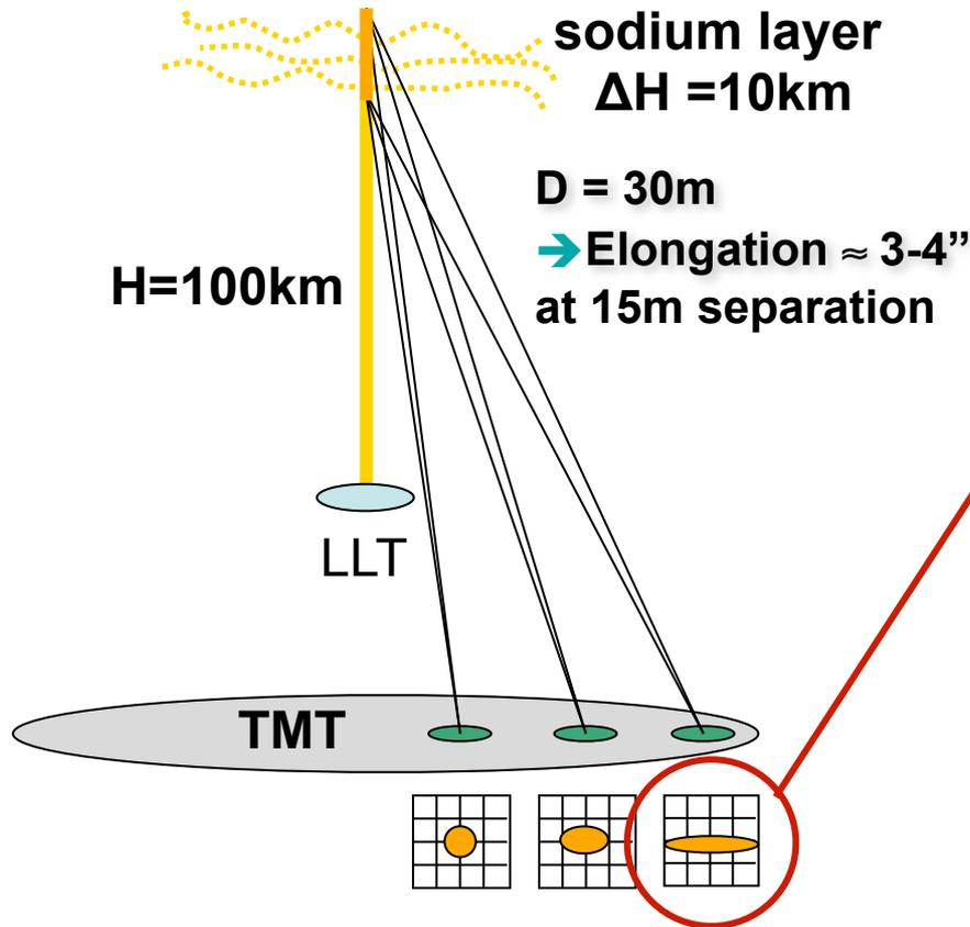
Fewer illuminated pixels than a large conventional CCD reduce pixel read rates and readout noise
