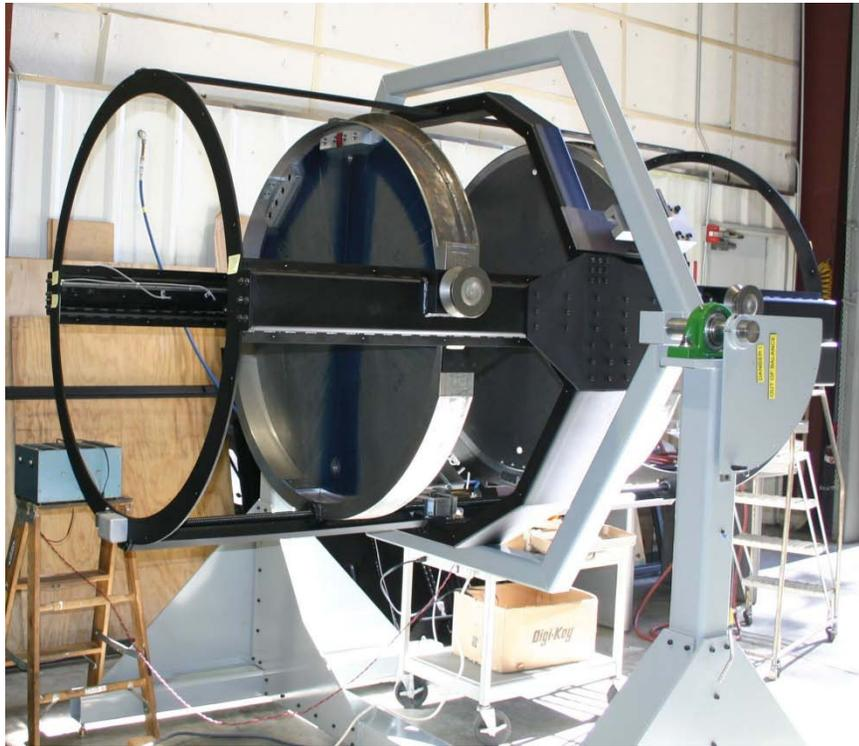
Keck ADC during fabrication at UCO – 1.0m prisms.
