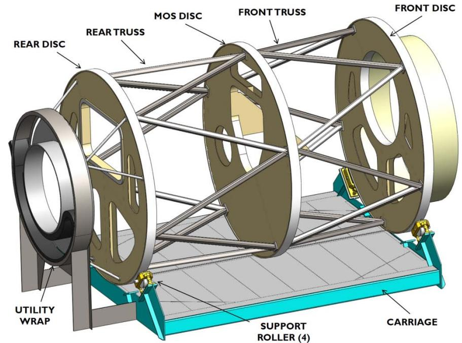
MOBIE structure and rotator – disks are ~4m in diameter.
