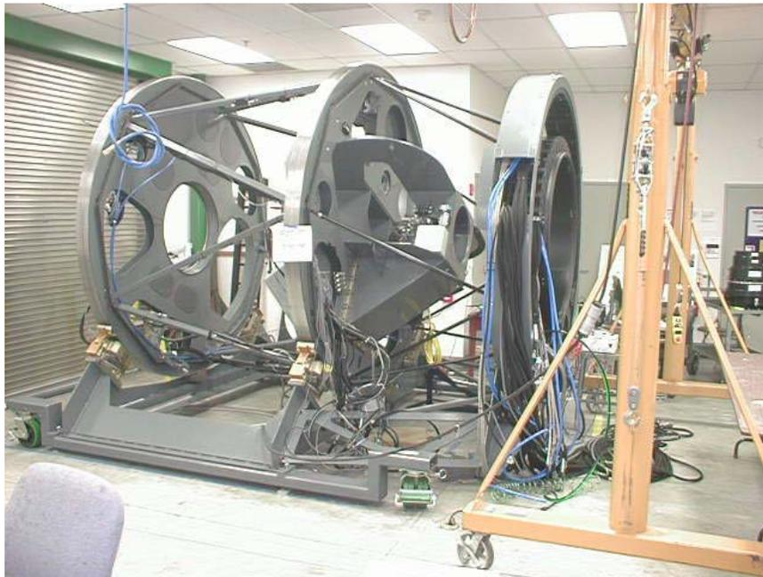
IMACS structure and rotator – disks are ~2m in diameter.
