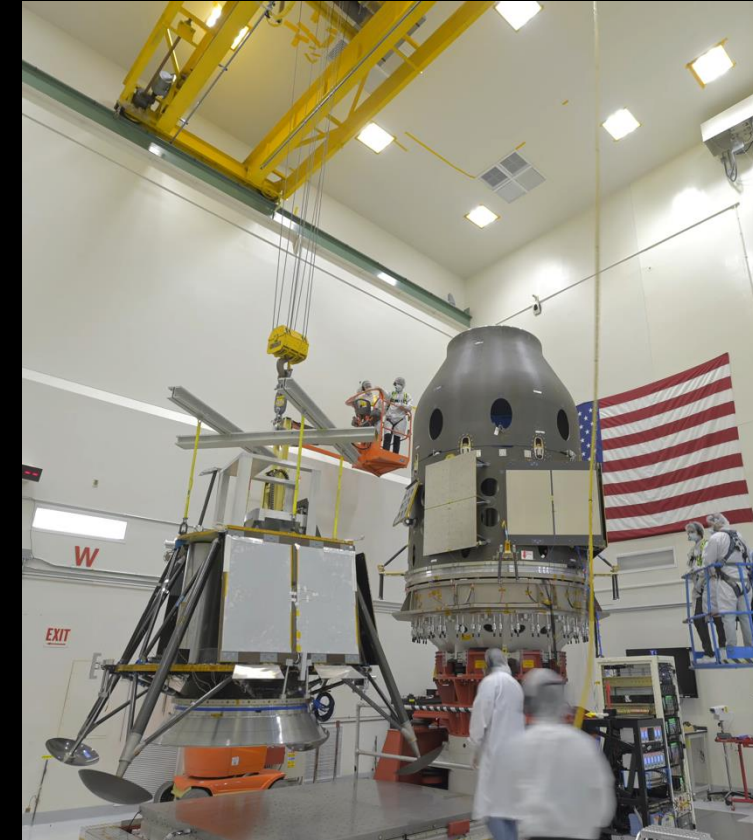
Assembly of Blue-Ghost 2 lander + orbiter at JPL prior to vibration testing
