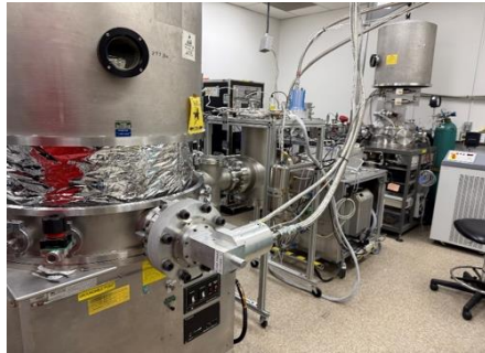
Test Setup for ^3\text{He} JT Stage Cooling Power Demonstration at 4.5 K
