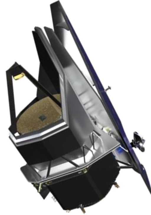
PRIMA Observatory with 4.5K Primary Mirror and 0.12 K MKID Detectors
