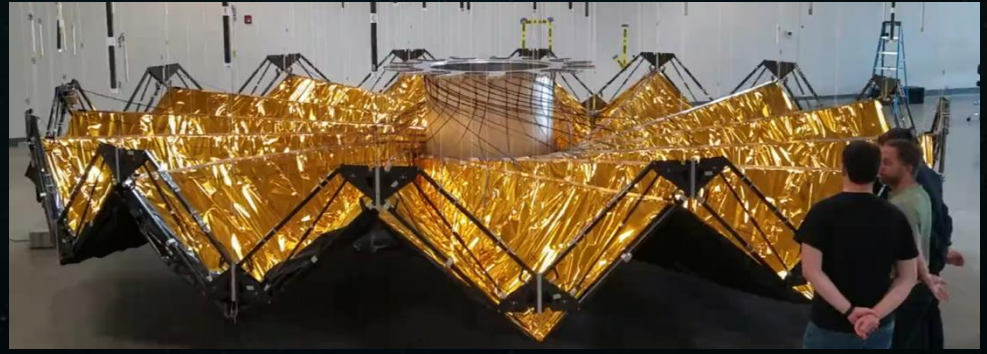
Stowed and partially deployed 10 m disk with optical shield
