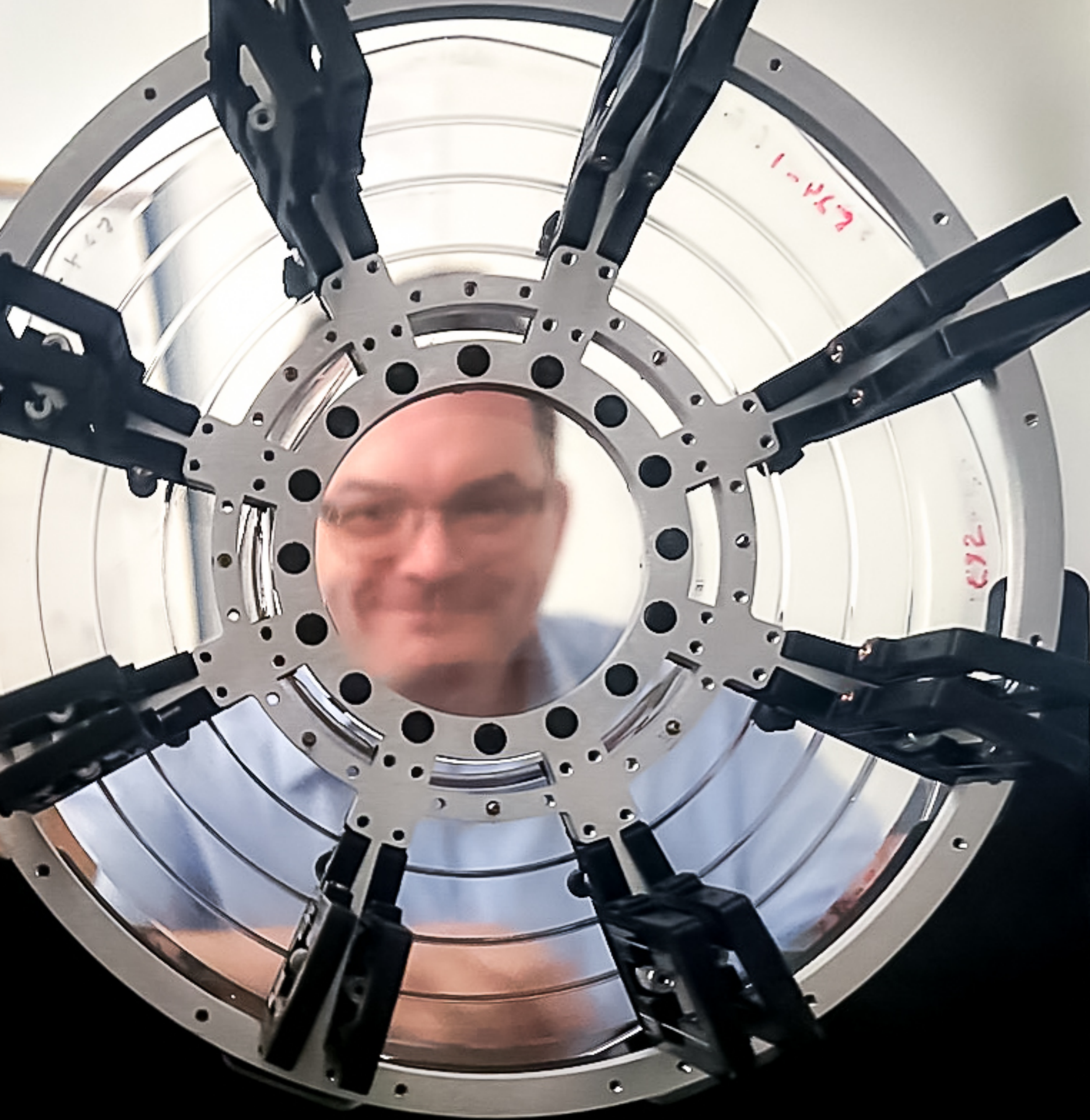
World's largest multi-order molded diffractive lens in alignment mechanism
