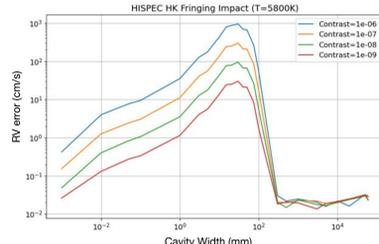
The fiber injection transmissive optics will be wedged to reduce the coupling of the coherent fraction of the ghosts. The goal is for the ghost to science contrast to be <3e-9 for each optic.
