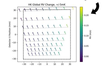
Thermal stability relative to calibration trace is 6 cm/s on average for 10mK peak-to-peak. HISPEC's goal is 1mK RMS stability, and more thermal analyses are planned.
