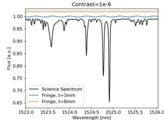
Fringe impact was simulated at the 1D level assuming variable etalon thickness, t
