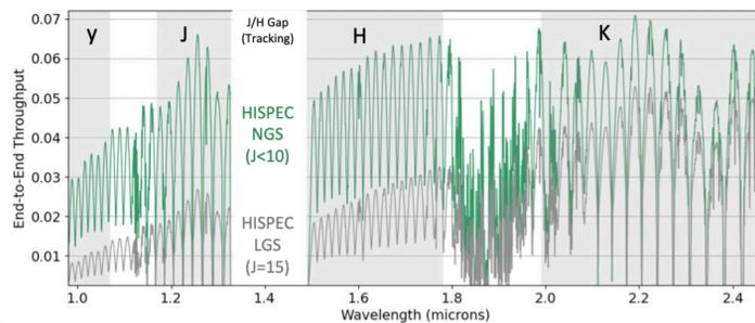
Throughput of HISPEC for natural guide star mode (NGS, using a Shack Hartmann) and laser guide star (LGS) at the faint limit of J=15.
