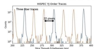
Cross coupling was estimated for using PyEchelle to be ~0.05% before alignment errors, which at most could double the value.
