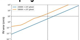
RV error versus the contrast of LFC cross talk relative to the extracted science light. We plan to reduce cross talk further in post processing.
