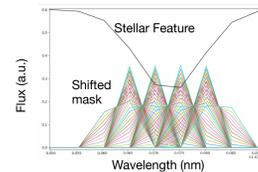
Stellar binary masks were generated from the Phoenix spectra themselves - these were cross correlated against the model spectrum before/after inducing spectral noise sources.
