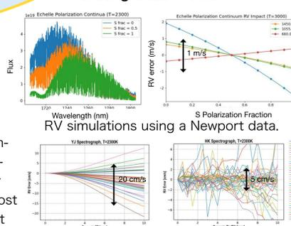
It is known uncorrected blaze changes leave m/s errors. HISPEC will blaze correct as the baseline correction, but is investigating polarization scrambling options. Other continuum changes (e.g. fiber coupling) show 5 cm/s post correction is possible, but more validation is needed.
