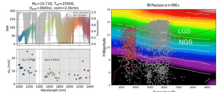
Simulated RV performance of TRAPPIST-1 assuming a 50 cm/s noise floor. The photon-noise limited RV precision follows the methods of Bouchy et al. 2001 masking tellurics >1% deep.
