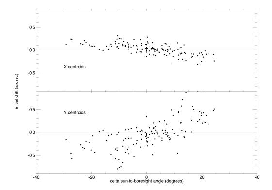
Initial x and y-pixel drifts in 118 exoplanet observing sequences vs. mean change in pitch angle for targets observed during the previous half hour.
