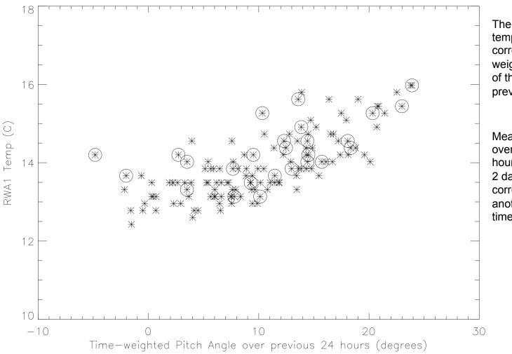
The RWA1 and RWA2 temperatures are strongly correlated with the timeweighed mean pitch angles of the telescope over the previous 24 hours.
