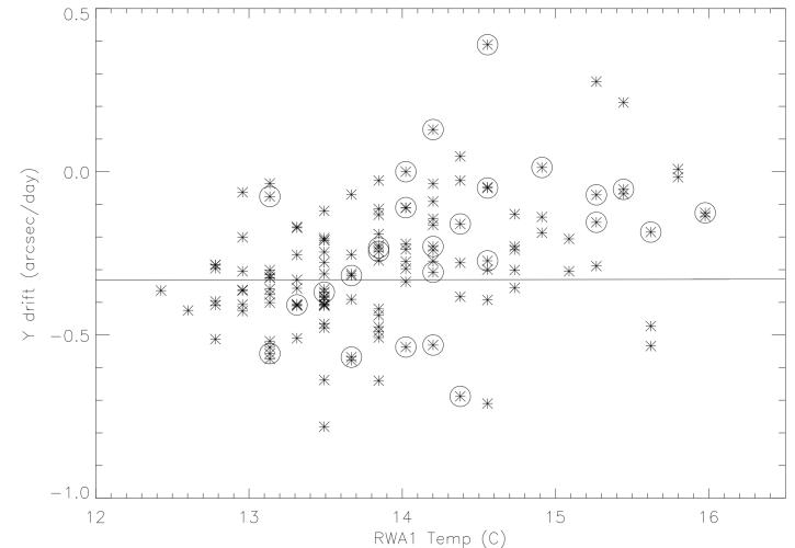
Y-pixel drift shows a rough correlation with the temperature measured at the RWA1 and RWA2 (but not RWA3) at the beginning of the AOR.
