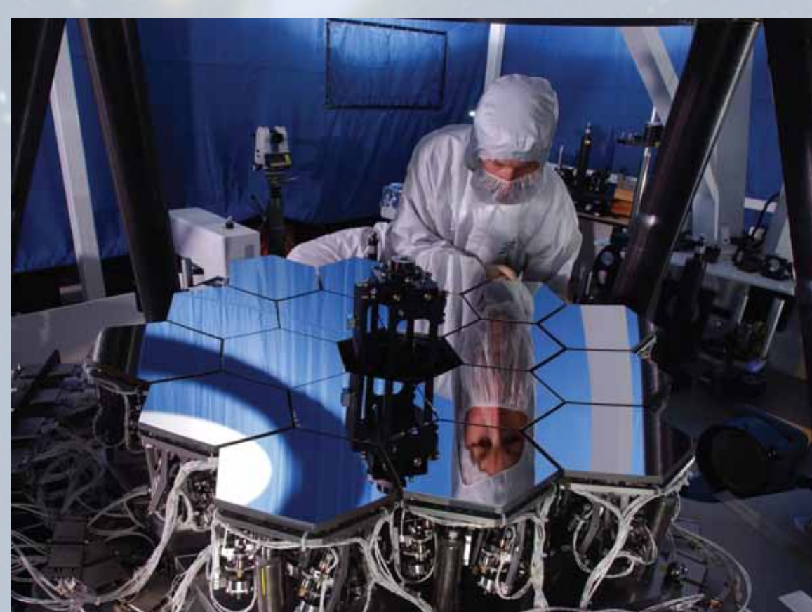
The Test Bed Telescope is a technology development program that matured the hardware and algorithms for phasing of the segmented primary mirror of the James Webb Space Telescope.
