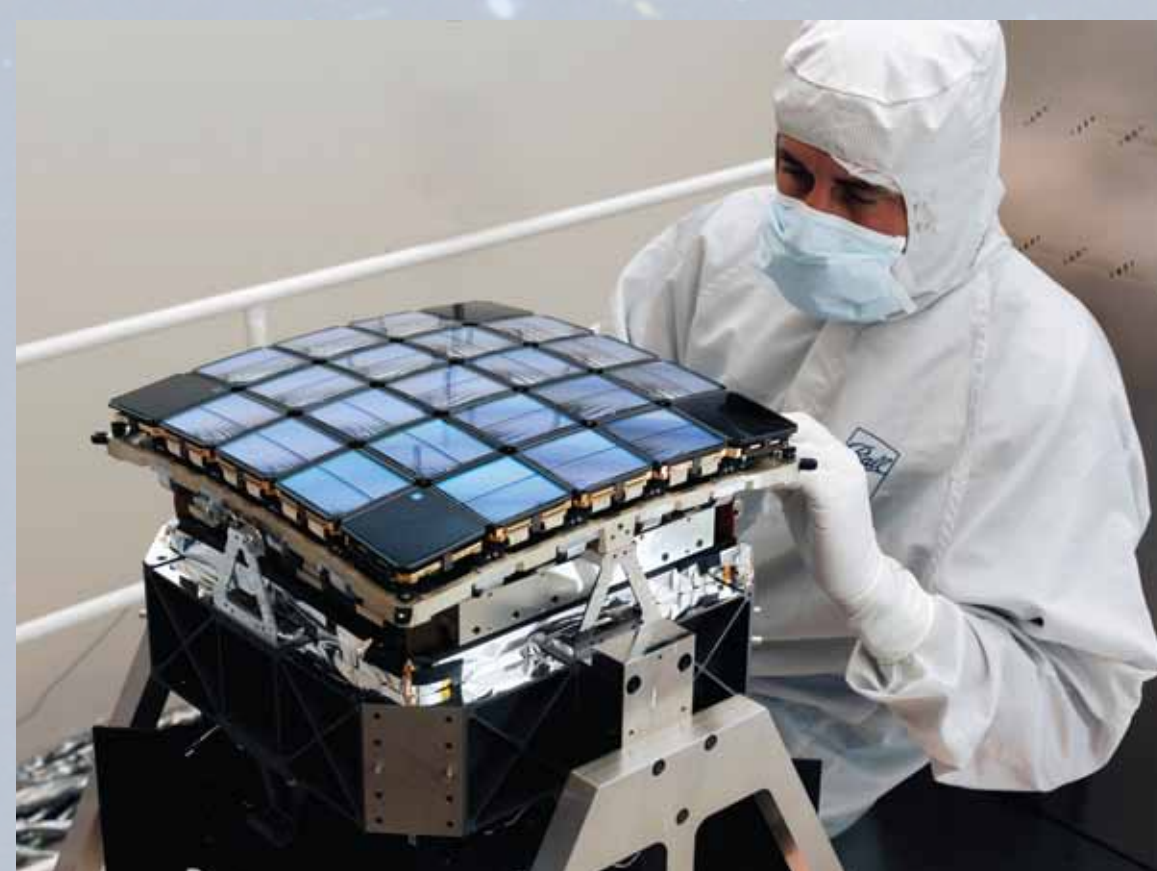
The focal plane array for Kepler is a mosaic of 42 CCDs assembled on convex substrate.
