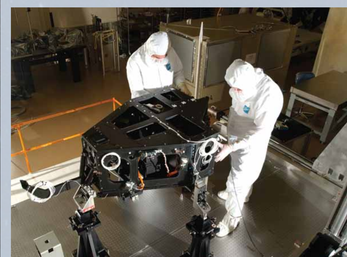
Wide Field Camera 3 is the primary UV/Optical/NIR imager aboard the Hubble Space Telescope.
