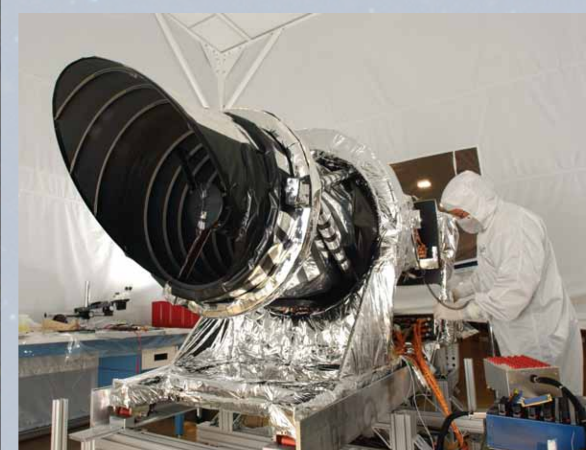
The HiRISE instrument undergoing final preparation. It is currently in space as part of the Mars Reconnaissance Orbiter.
