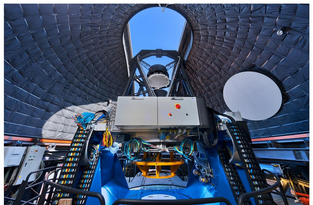
PS2 telescope w/ optics assembled inside PS2 dome on Haleakala.
