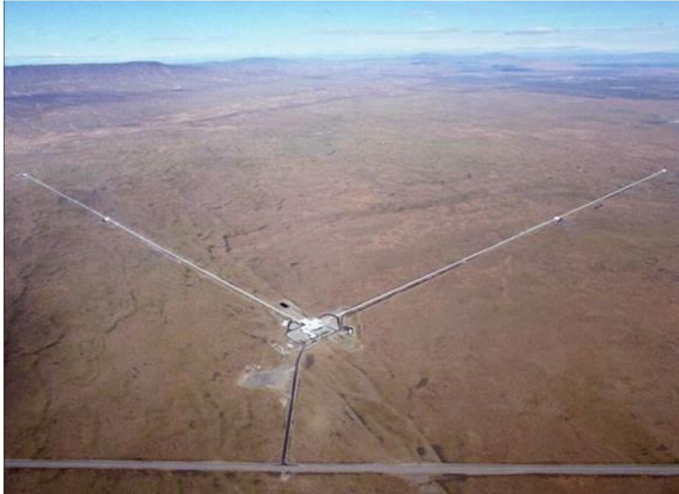
Advanced LIGO will be able to detect gravitational waves that stretch the length of the 2k arms by a fraction of the size of a proton
