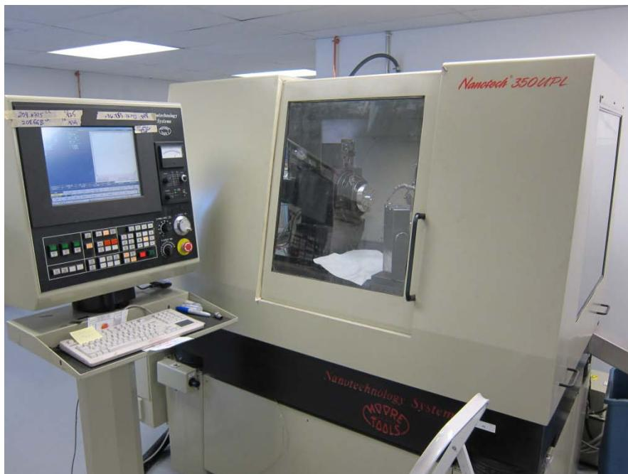
One of two diamond turning machines at Optical Solutions Inc.
