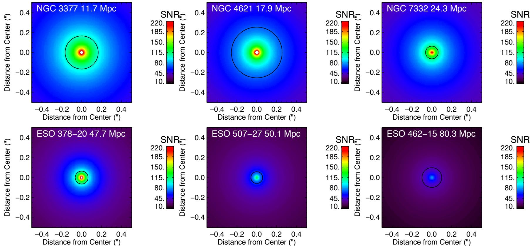
Simulated average S/N per spectral channel at 9 mas plate in  $K$  band with eight observations of 900 s each (2 hr integration time) at  $R = 4000$ .
