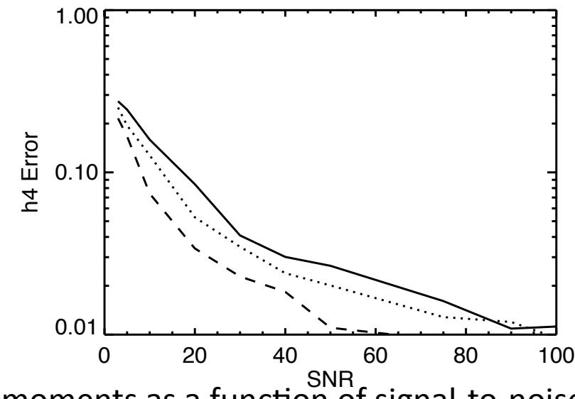
Errors in Gauss-Hermite moments as a function of signal-to-noise ratio
