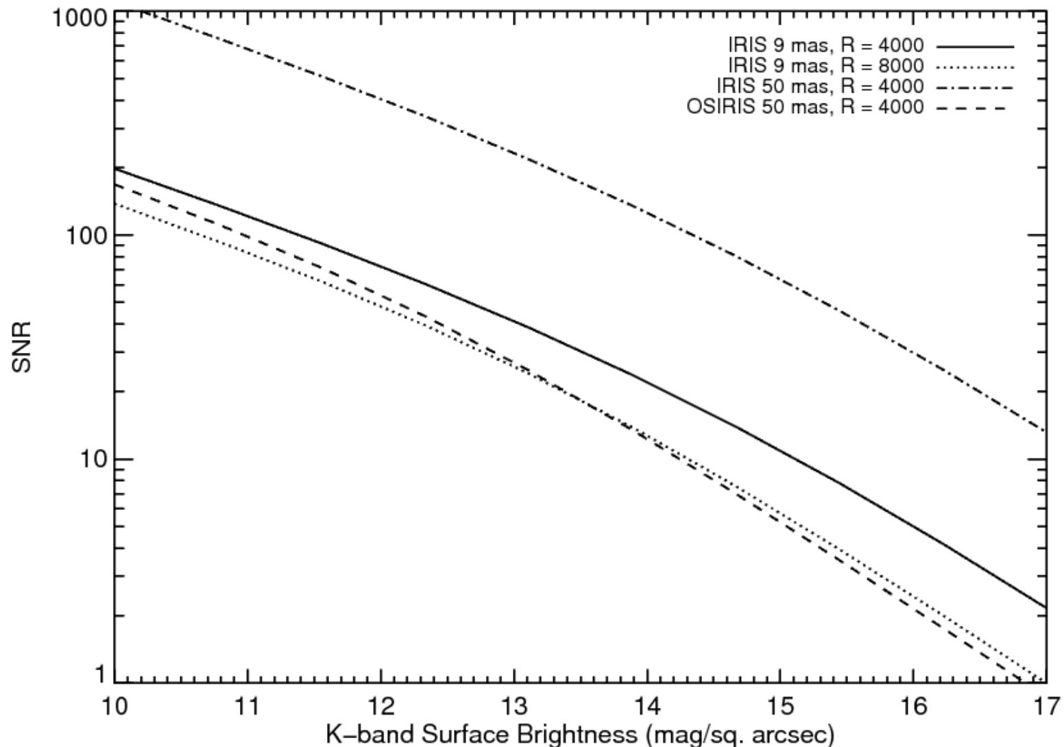
Ave. SNR over K-band for 5 hours of integration time (20x900 s exposures)
