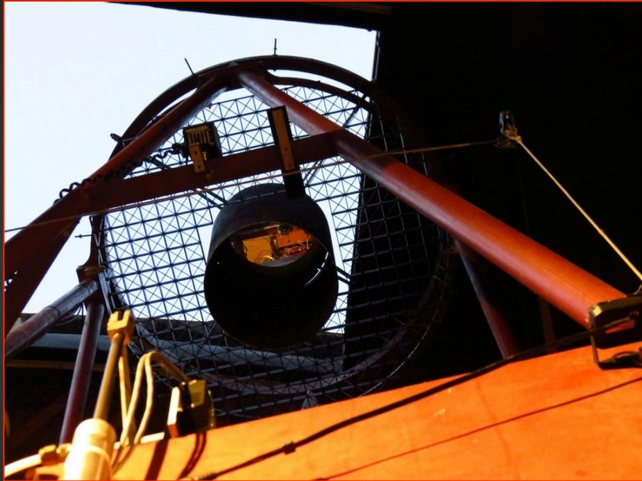
Carbon mask installed on Nickel Telescope (Credit: E. Bendek)
