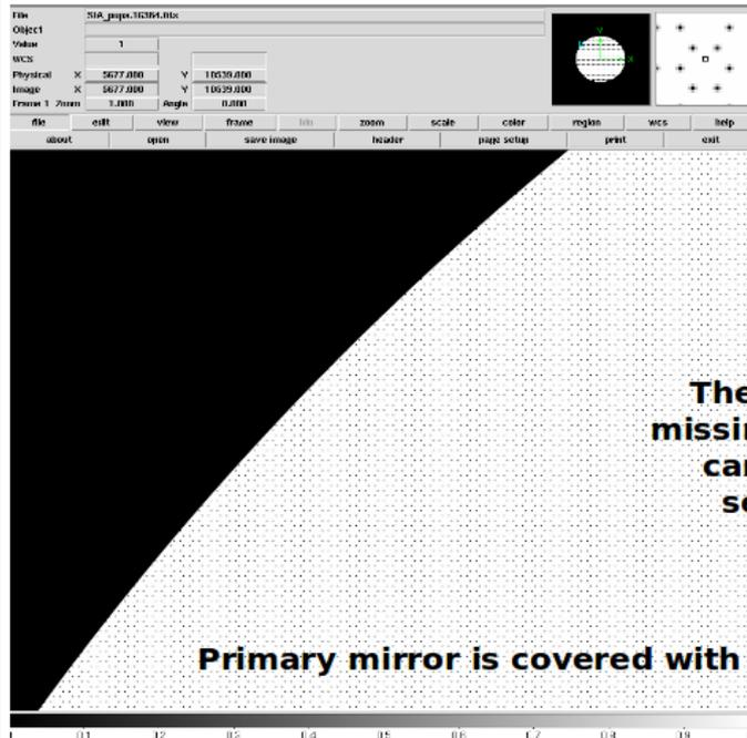
**The center of the field is missing from the astrometric camera (central light is sent to coronagraph)**
