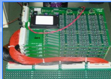
DM Electronics Prototype & CILAS DM 6x60 Breadboard test setup (warm) at NRC - Herzberg
