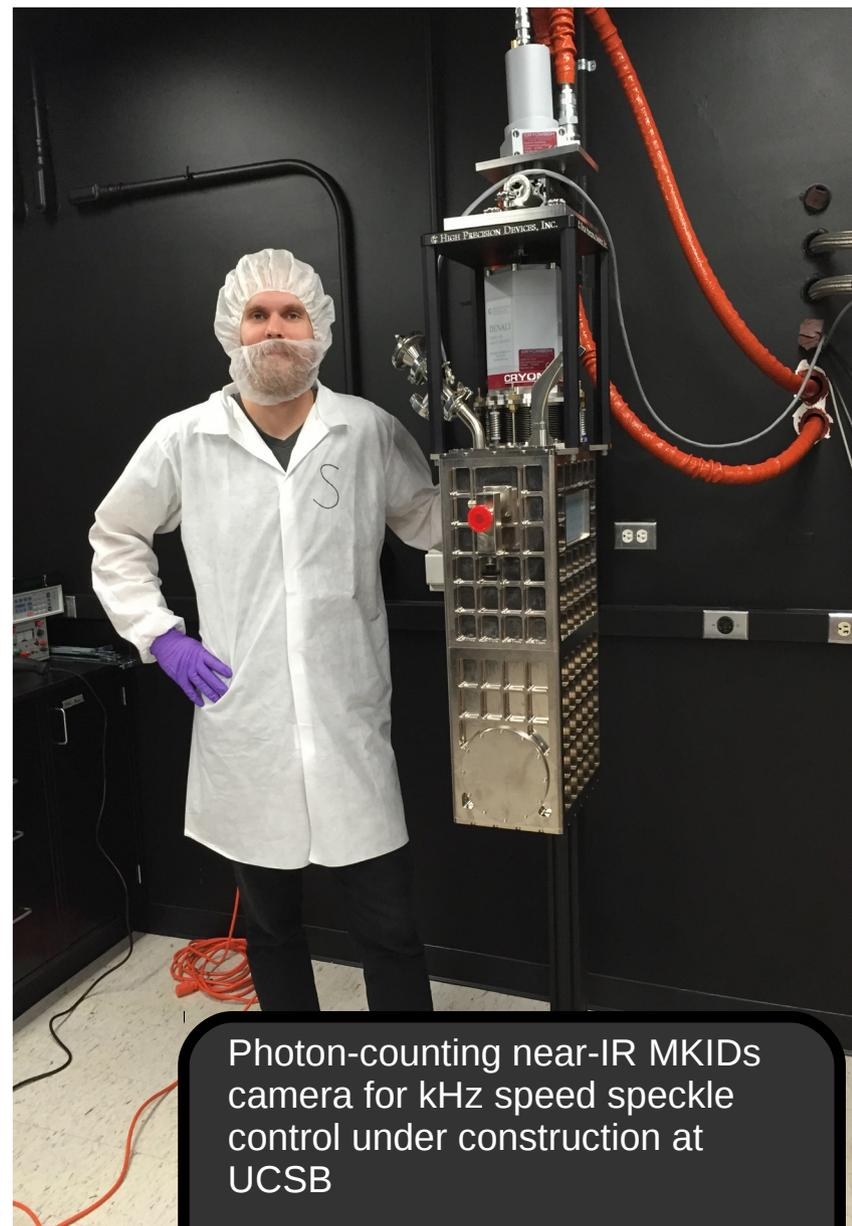
Photon-counting near-IR MKIDs camera for kHz speed speckle control under construction at UCSB
