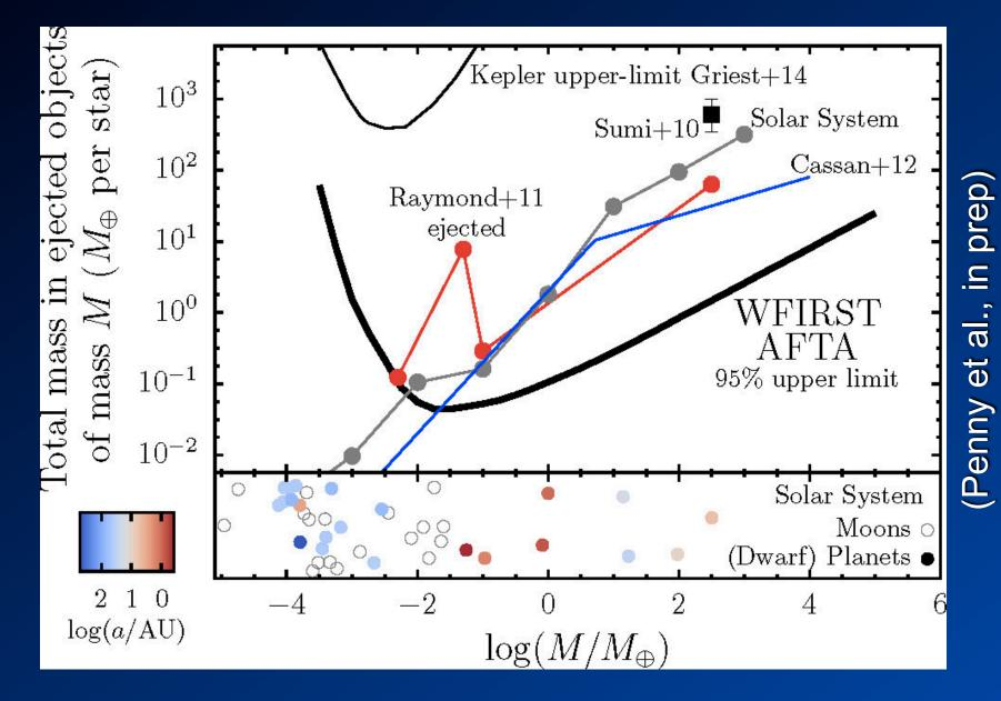
WFIRST-AFTA will measure the compact object mass function over at least 8 orders of magnitude in mass (from Mars to ~30 solar masses).
